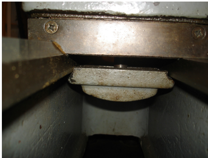
Figure 195: Tailstock anchor in position under bed.
