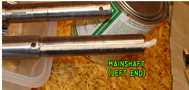
Figure 141: Mainshaft showing new felt.
