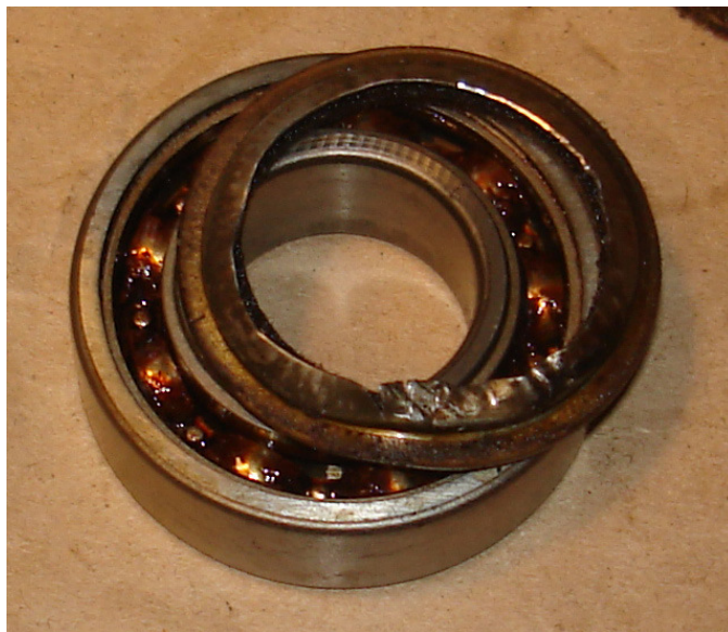
Figure 17: Failed countershaft bearing with shields removed.
