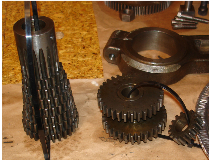
Figure 135: Gears stacked to preserve orientation.
