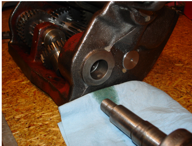
Figure 146: Reinstalling the leadscrew in the gearbox.
