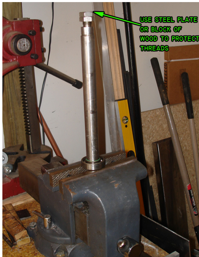
Figure 18: Pressing on the first countershaft bearing using a bench vise.
