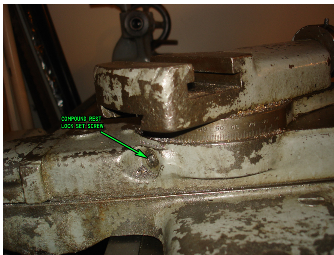
Figure 102: Compound rest lock screw. There is a second one on the other side.
