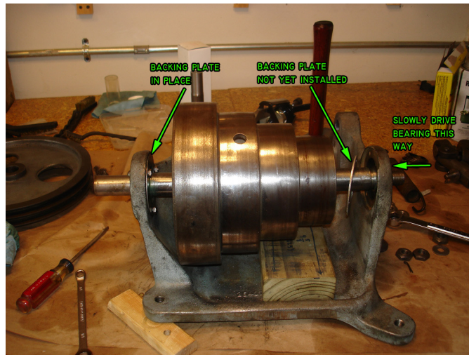
Figure 20: An interim step in installing the cone pulley.
