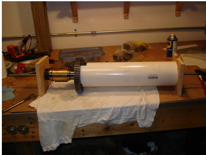
Figure 57: Bull gear being pressed on.
