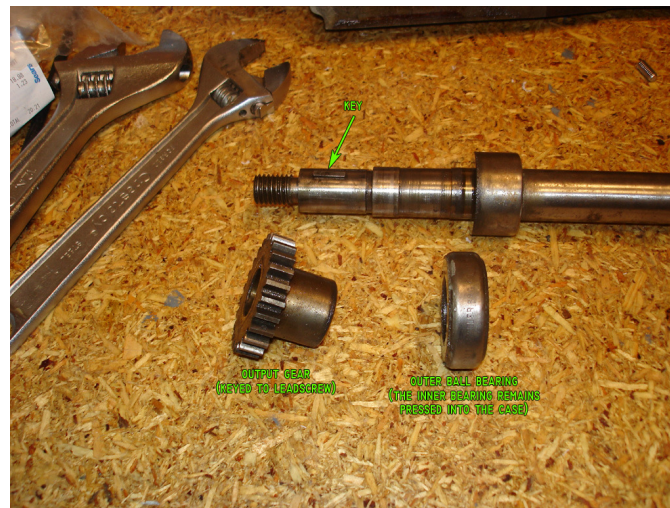
Figure 127: Detail of leadscrew where it enters the gearbox.
