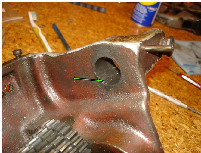
Figure 132: Shift rail hole showing felt wick.
