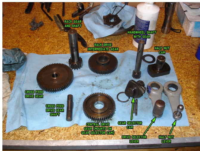
Figure 167: Complete apron gearset layout.
