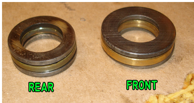
Figure 117: Front and rear cross slide leadscrew bearings.
