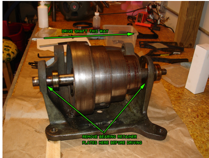
Figure 12: How to remove the underdrive pulley assembly.
