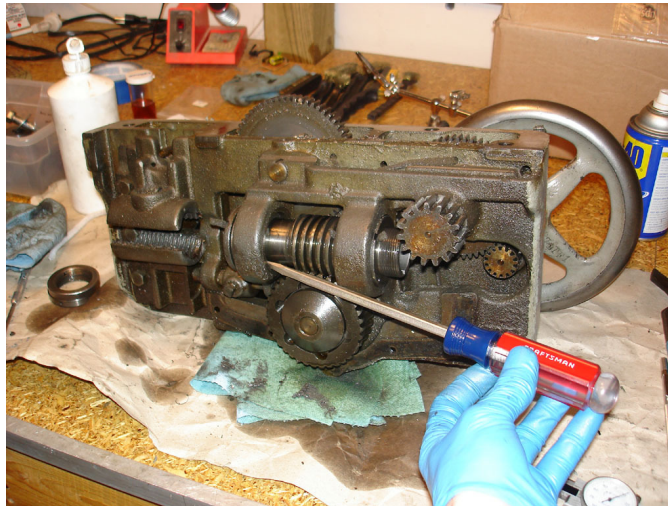
Figure 156: Driving out the worm drive end caps.
