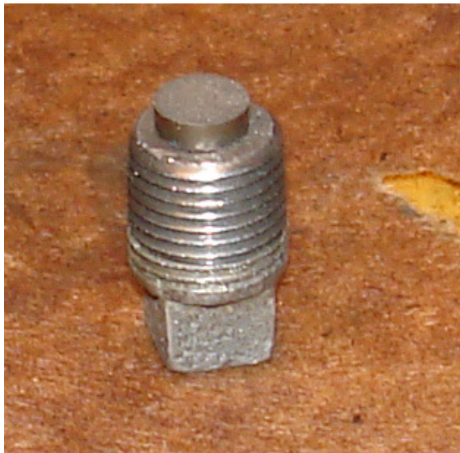
Figure 185: Magnet on apron oil drain plug.
