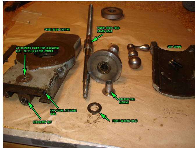
Figure 118: Complete cross slide in pieces.
