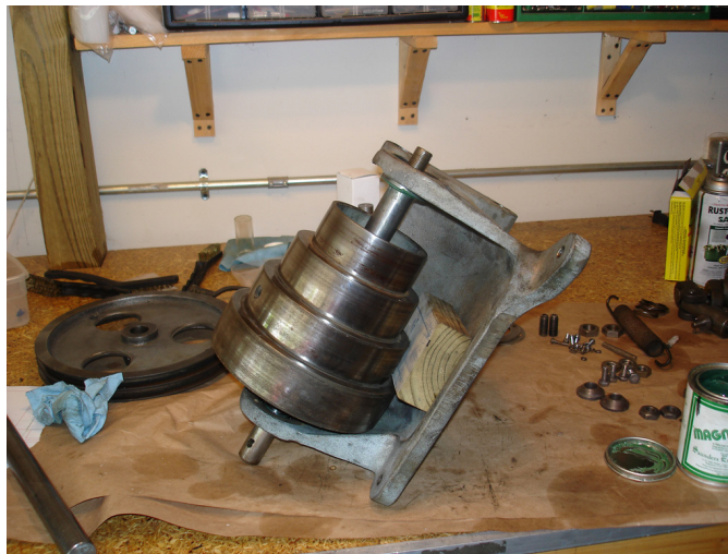
Figure 21: A method for supporting the left end of the countershaft while the right side bearing is pressed into place.
