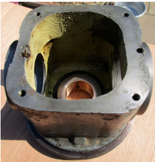
Inside head casting. Drive pinion bronze bearing in place.
