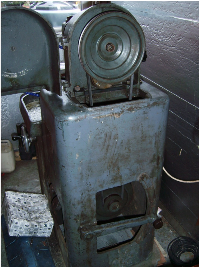
Rear view set up in direct drive high speed range.
