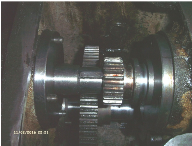
Shows drive key with small gear disengaged
