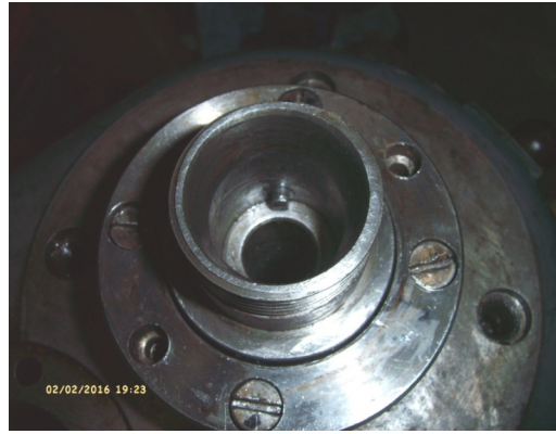
Front end view of assembly. (Shows drive key)
