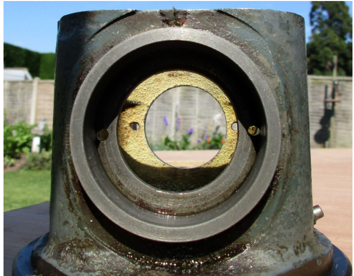
Bottom bearing c'bore. (2 small holes to extract outer race)
