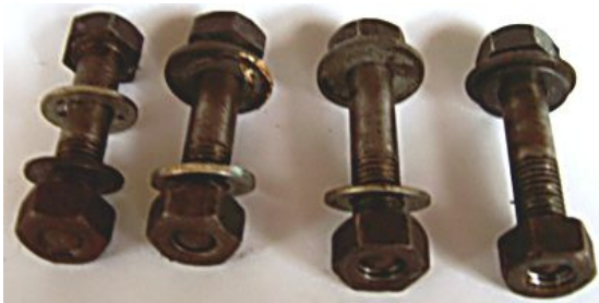
Mounting bar bolts: 1.5"longx5/16"BSFx.65"threaded
