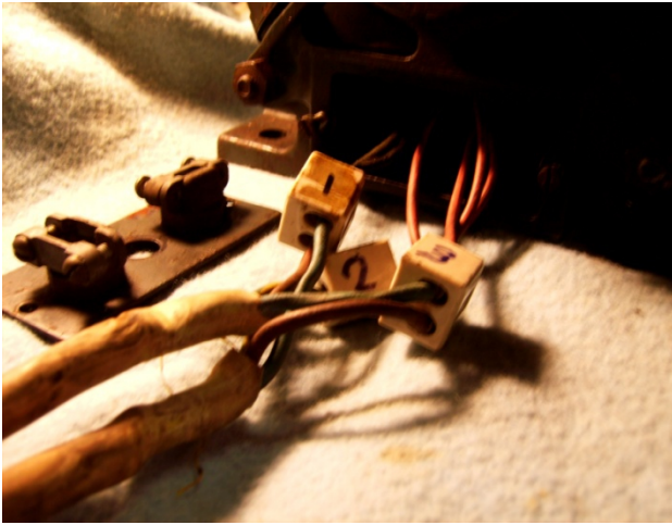
Ceramic connector blocks with test wiring connected.
