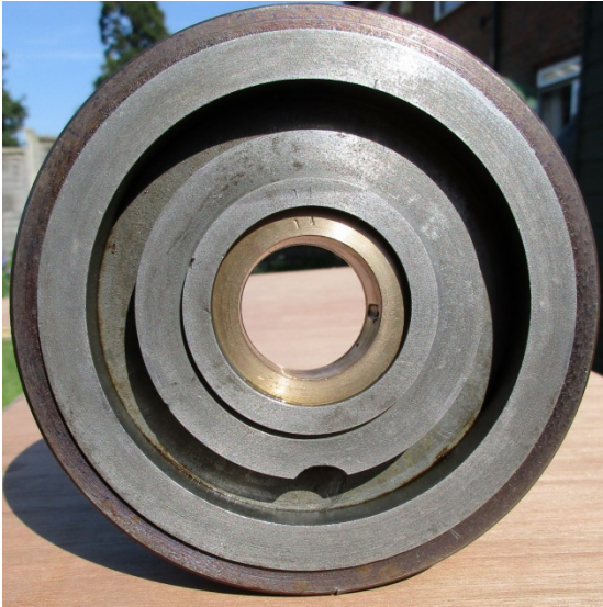
Rotating Head Mounting Face. Cutout for special T'bolts.
