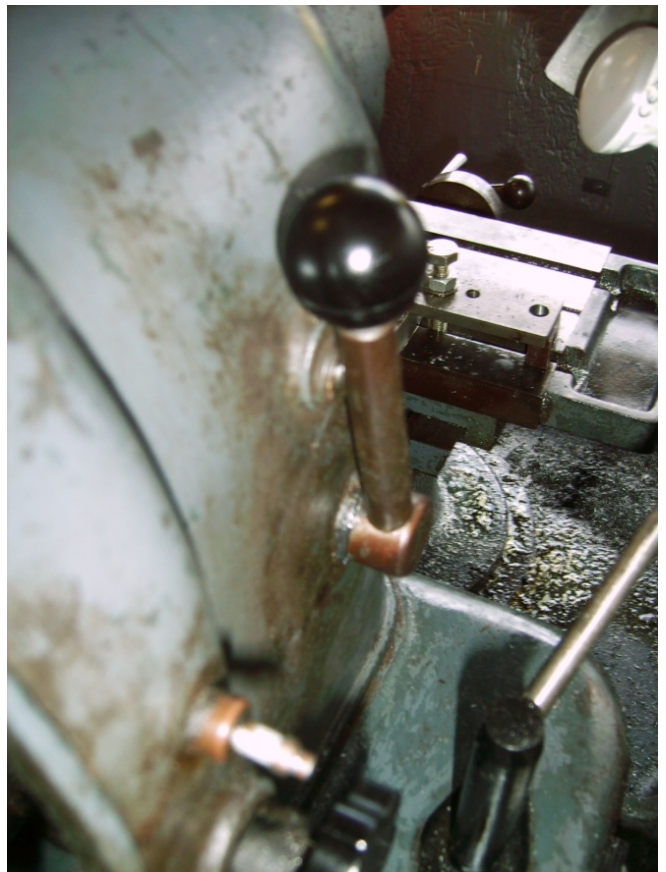
Position of side change over lever with back gear disengaged.
