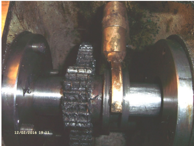
Picture of gear change assy. in place. Engaged position.
