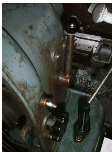
Shows change over lever in back gear position 2
