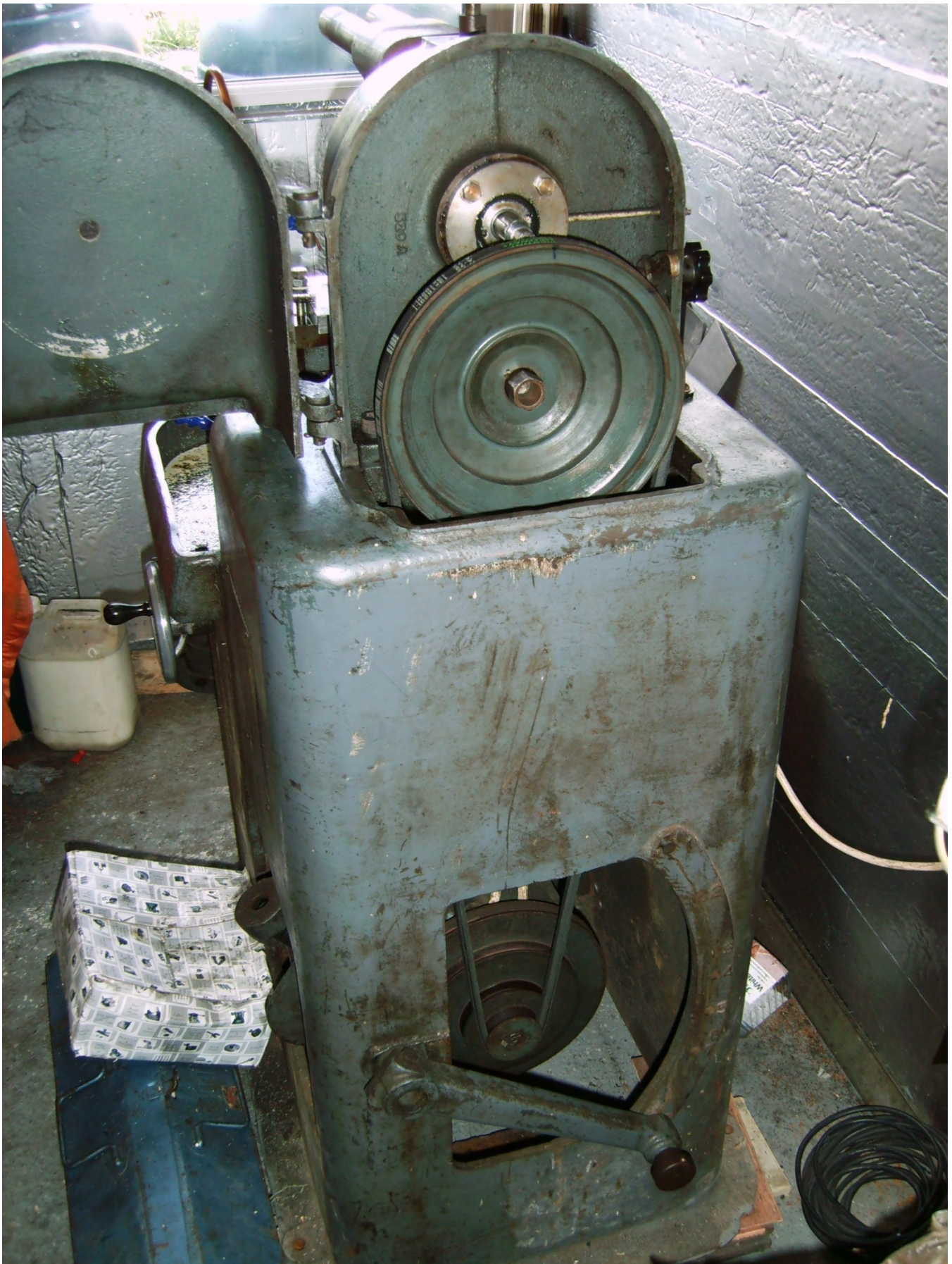
Shows rear view in back gear with machine set at slowest speed. Note: belt tension lever set at No.8 (lowest of 8 positions) position.
