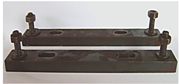
Motor mounting bars(slotted for adjustment)
