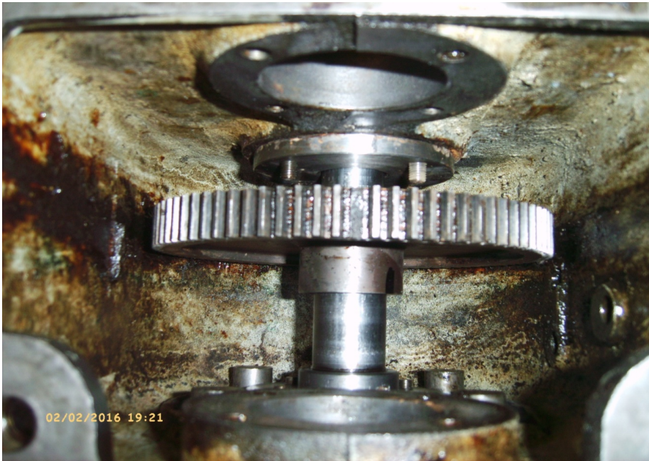
Picture of main shaft assembled in head casing.
