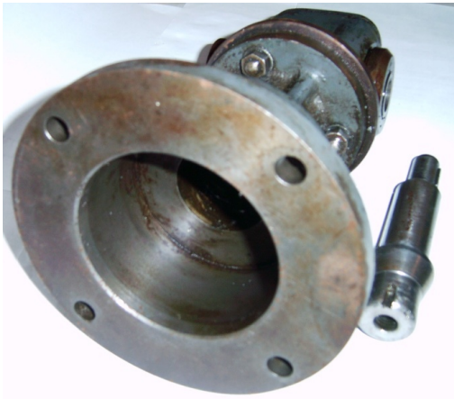
accessory mounting flange. Locates over front bearing housing.
