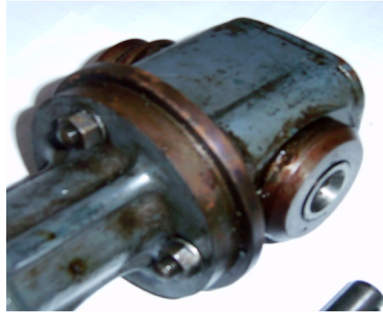
View of indexing part of head. 2 of clamping bolts visible.
