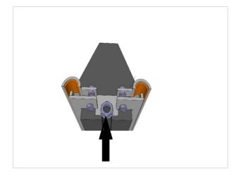
A long nut or handwheel should be added here.
