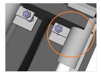
An overhead view of an externally-mounted way clamp.
