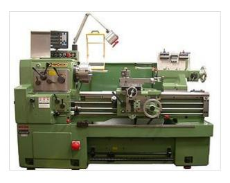
A metal lathe or metalworking lathe is a large class of lathes designed for precisely machining relatively hard materials. They were originally designed to machine metals; however, with the advent of plastics and other materials, and with their inherent versatility, they are used in a wide range of applications and a broad range of materials. This is a 100-year-newer, industrial version of the type shown below but this one, ours and the one below all work in exactly the same way.
