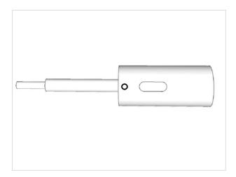
The spindle could be a solid Morse taper socket that has been drilled to accept a pinned shaft that has been turned down on the end to fit the drill chuck.
