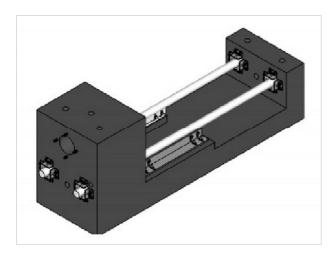
Insert the ways and lightly clamp in place. The supports under the ways are made from angle iron and steel bar. A longer lathe (recommended) should have full length way support. Round lathe ways will both sag and vibrate but a rigid support like this is a simple cure. After the machine is complete, the adjustment devices that are bolted to the concrete could be removed and used to build another lathe.
