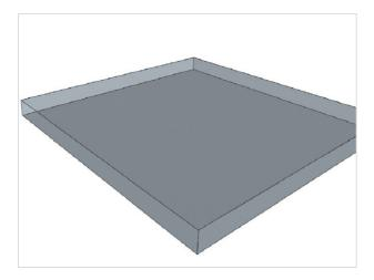
Consider the thickness of a thin piece of paper as an accuracy goal. Use a thick, square piece of plate glass (float glass is best) laid across the ways to check (with a feeler gauge) for even contact on all 4 corners. Rotate the glass and check again (the glass plate may not be perfectly flat). Move the glass plate from one end of the ways to the other to make certain everything is correct. Adjust the way supports for even contact under the ways.
