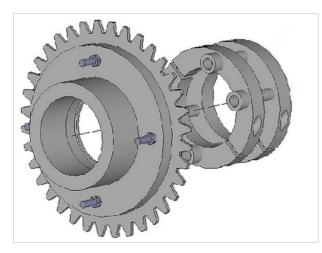
Temporarily, the adjuster could be replaced by the sprocket hub if a steel washer was used between them.
