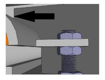
Close in the edge of the form here. Use the widest possible carriage width to support the base of the cross slide.
