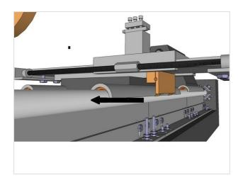
Steel for the ways will probably require a careful search. Needed are (2) 40mm x 1.5 meter (approx) very straight steel rods or pipes (scrap hydraulic cylinder piston rods? ) Check them for straightness by putting the round bars or pipe side by side and shining a bright light between them as you first rotate one, then the other.
