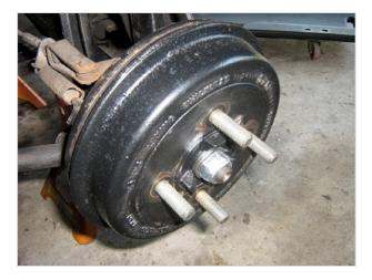
This is typical of a drum brake setup used on many vehicles. The drum will come off the spindle without too much trouble in many cases. Reverse the drum, add screws (for jaws) and a simple 3- or 4-jaw "cup chuck" can be made. As with the prior spindle design, while it is far from perfect it will work to make parts and train operators. Machining pressure plates, brake rotors, etc. does not need a hollow spindle.
