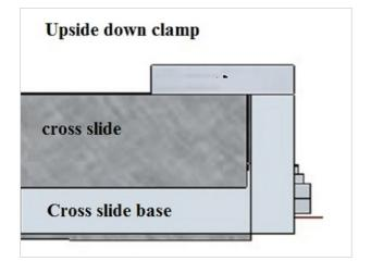
Another way to build machine slides is to invert the clamp. This lets you build the cross slide assembly using just two pieces of steel of the same width. This may be more economical and in some areas might be the only way practical. The disadvantage is that metal particles from machining may get between the clamp and the slide. Leather wipers attached to the edges of the top pieces of the clamp should help with this. Wear could be adjusted for by judicious filing or adding a thin shim.
