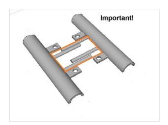
Using a pre-cast, seasoned concrete bed is critical to the project and SO is the steel frame for the carriage. Most machine builders would find it difficult to build a welded or bolted carriage frame that would have the vital even contact on the ways. We avoid the problem by making the frame in 2 pieces, clamping them to the ways, and then using concrete to fix the 2 sides in place permanently.
