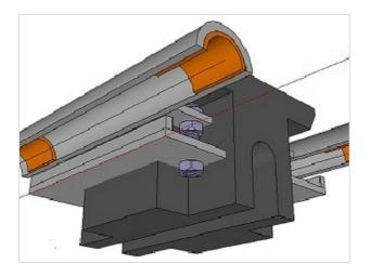
On a carriage for a lathe with shorter ways.space saving techniques must be used. These clamp bolts fit into notches cast into the carriage. A longer carriage will be easier to make because the clamps can be external and the inner parts not so crowded together.
