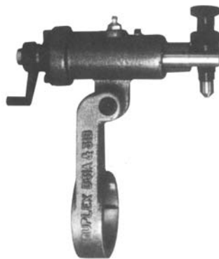
The BUILT -IN DIAMOND DRESSER IN POSITION
